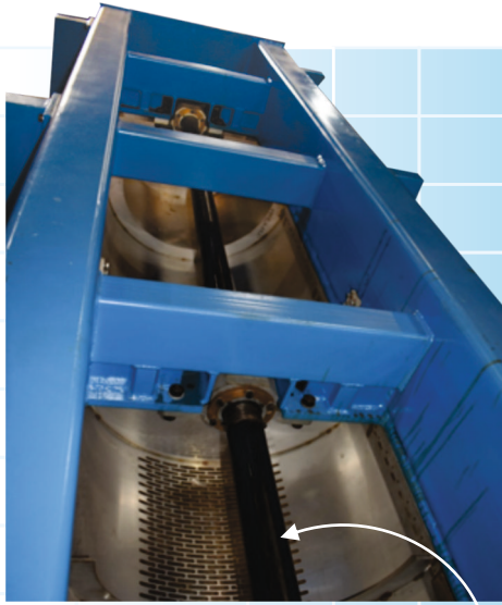
Boring bar holding tool at Baffle position
